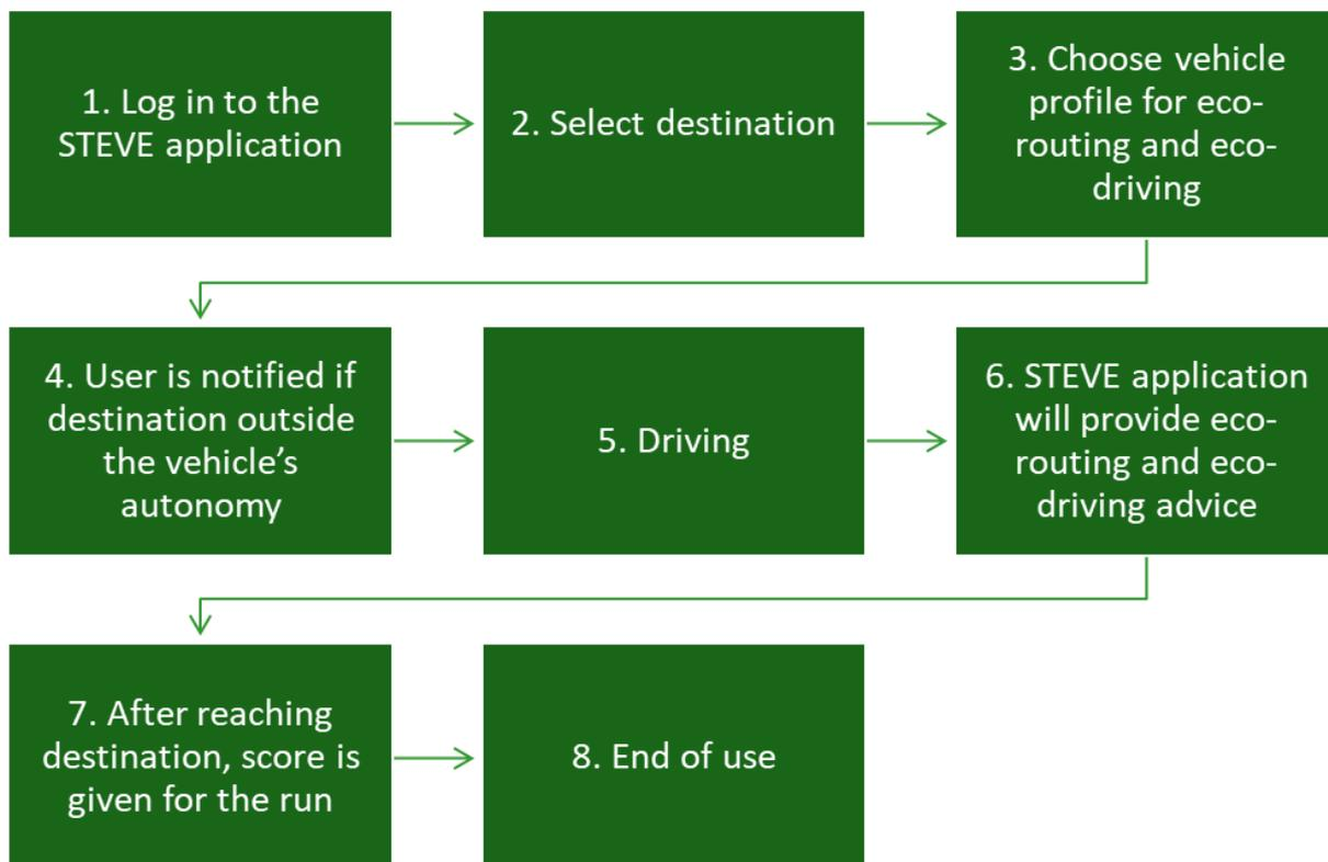
Fig 2. User-centric process diagram of STEVE Eco-driving use cases.
